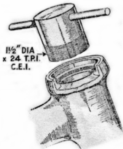
Fig. 42. Steering head ballrace extractor.
