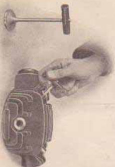
Illustration 4. HOW TO USE THE A.S. VALVE GRINDING TOOL.
